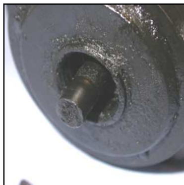
Turbo shaft failure
